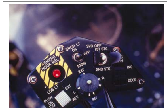
Figure 7. Note how the switch guard and landing light adjustment switch correspond to the injuries of the pilot.
